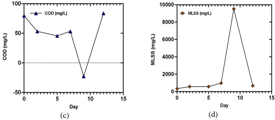
Figure 5. Operational parameters of synthetic wastewater (a) relationship between SVI and MLSS (b) pH and SVI overtime (day) (c) COD overtime (day) (d) MLSS overtime (day)
