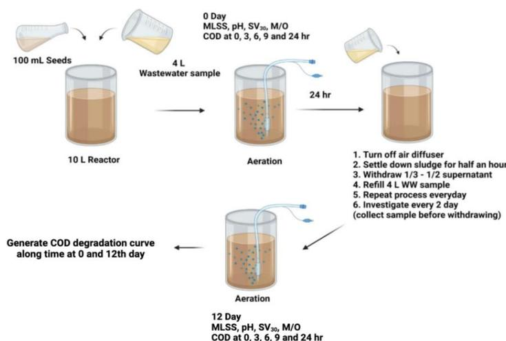
Figure 1. Aerobic degradation test
